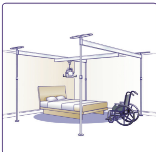
The 4 post Easytrack operates like a traditional x-y system covering all 4 corners of a room. The 4 post is not telescopic.
