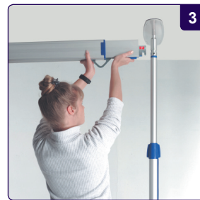
Extend rail to required length and fix rail onto second post.
